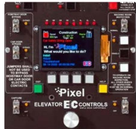
To make sure that all of the pieces work together properly, a CANbus communication system has been designed into the Pixel system (CAN = Control Area Network). CANbus technology has
